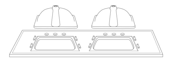
2. Apply a continuous bead of sealant to the top surface of the sink's rim, where it will come into contact with the underside of the countertop.
