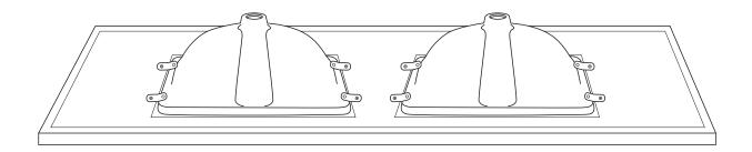
4. Two people, three for double sink tops, must lift the countertop (A) and carefully place it positioned on top of the vanity base (D). See page 4 for more details.
